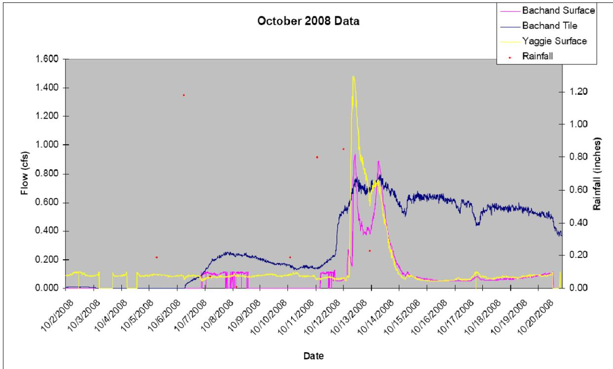
**Figure 68. Example runoff event hydrograph showing peak flows (before normalization)**
