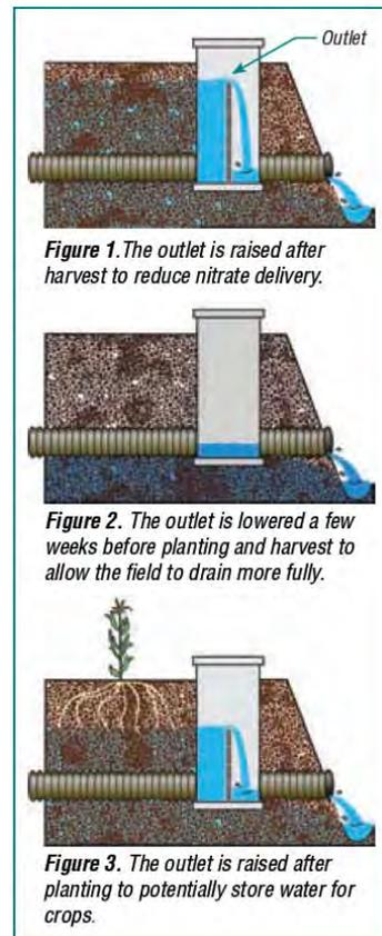
**Figure 1.** The outlet is raised after harvest to reduce nitrate delivery.
