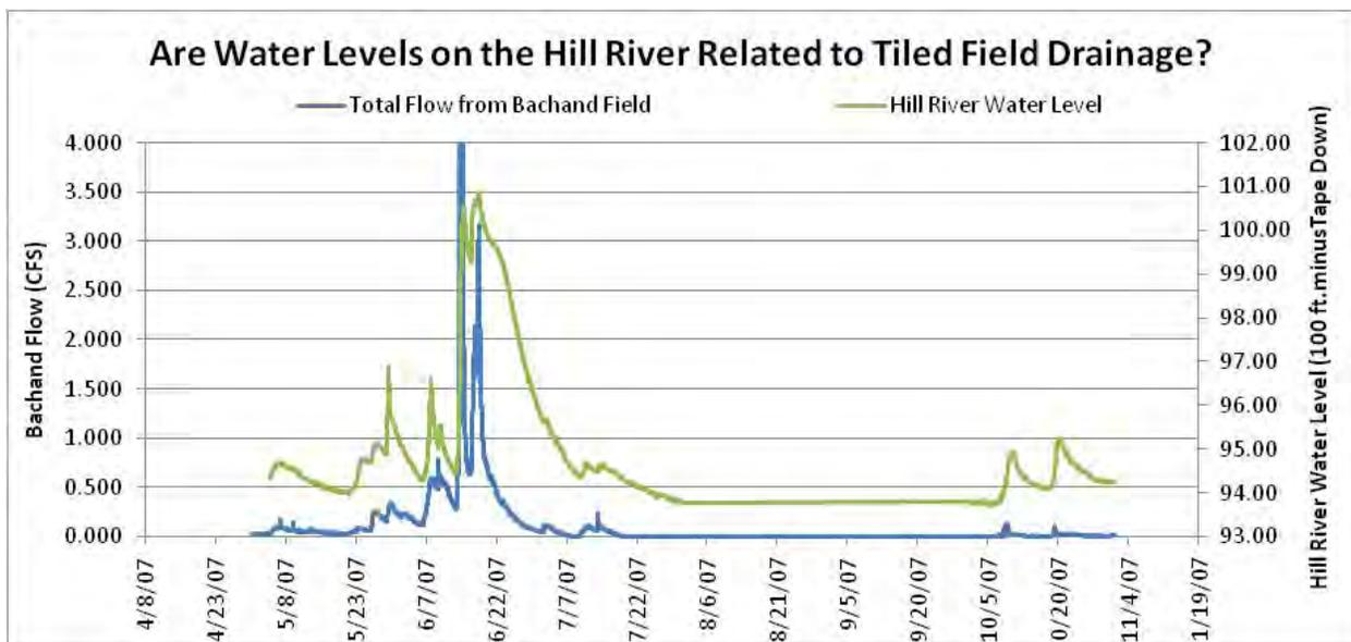
**Figure 76. 2007 Hill River Water Levels and Tile Flow Rates**
