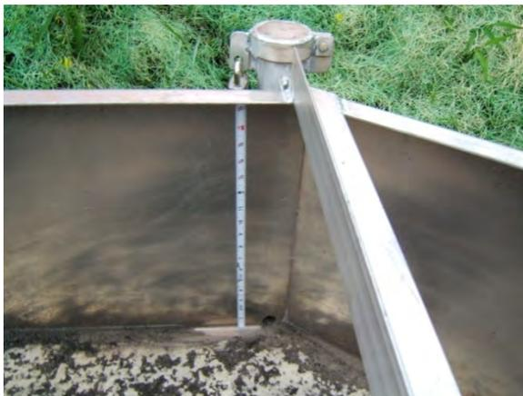
The site is affected by backwater from the Hill River. A decision was made to raise the structure after the 2007 monitoring season in order to continue monitoring and have more confidence in the data. This was accomplished in the spring of 2008 and successfully maintained a level of head above the tail-water and reduce erosion.
