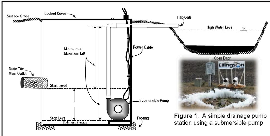
**Figure 1.** A simple drainage pump station using a submersible pump.
