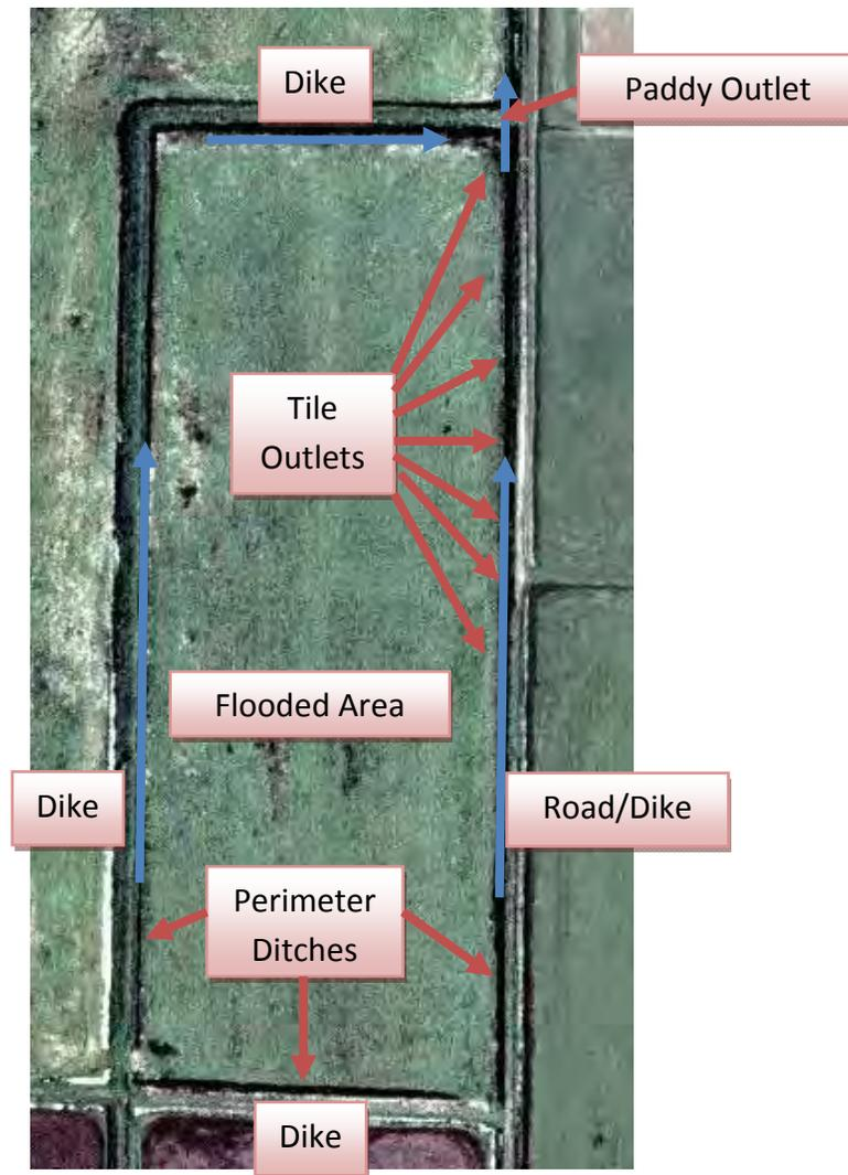
**Figure 10. Diagram of a tile drained field with internal perimeter ditches.**
