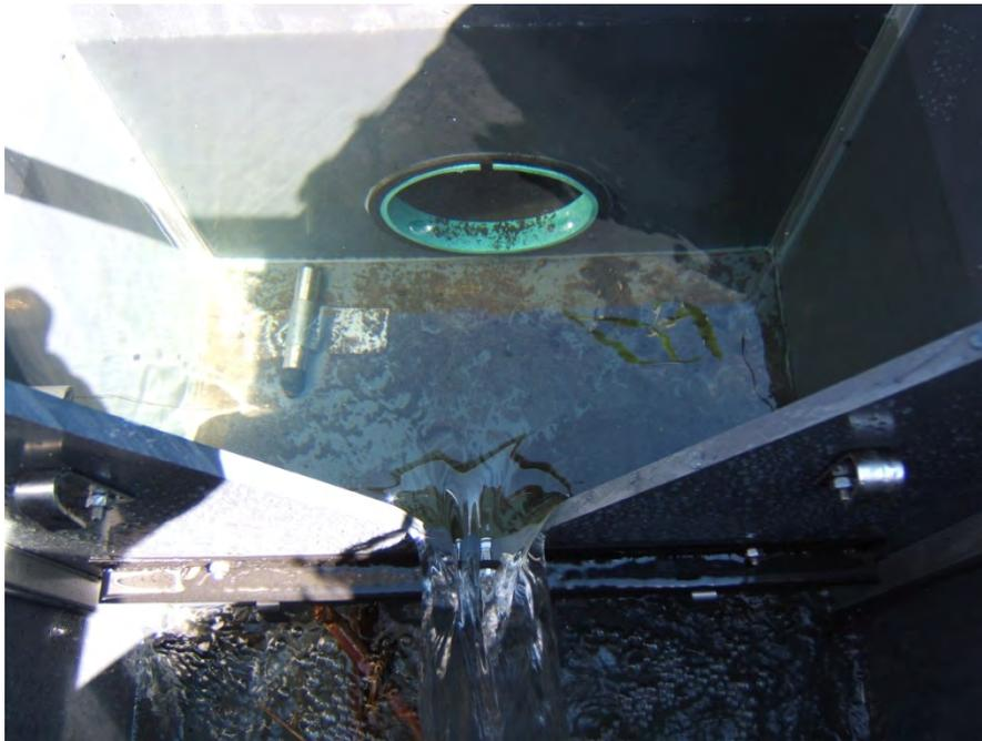
**Figure 13. V-Notch Weir and HOBO Water Level Data Logger in the Bachand Water Control Structure**
