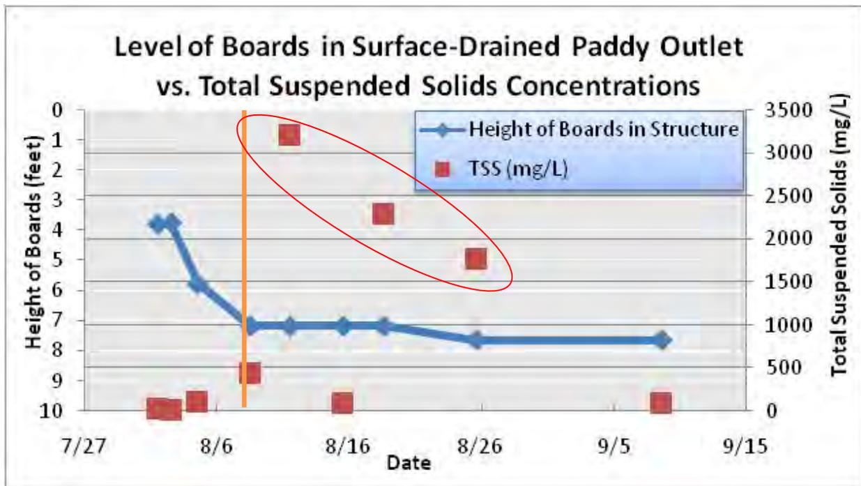
**Figure 40. Water quality problems at the surface drained paddy outlet began when nearly all of the boards were removed from the structure.**
