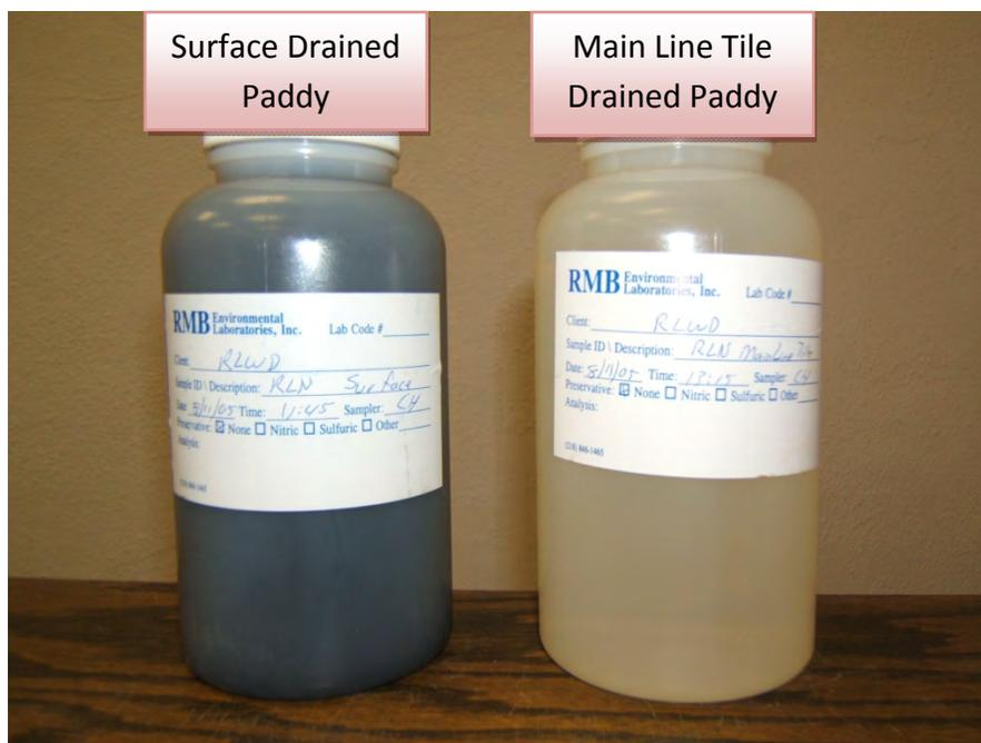
**Figure 41. Wild rice paddy surface drainage and main line tile water samples.**
