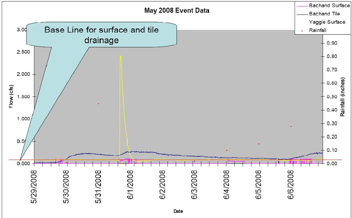
**Figure 70. Finding the base line flow for each runoff event**
