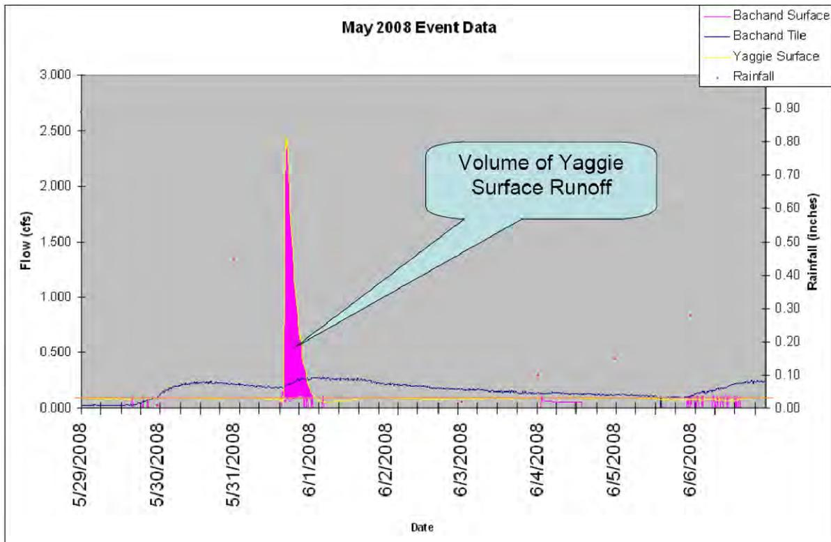
**Figure 72. Calculating runoff event flow volume for surface drainage**
