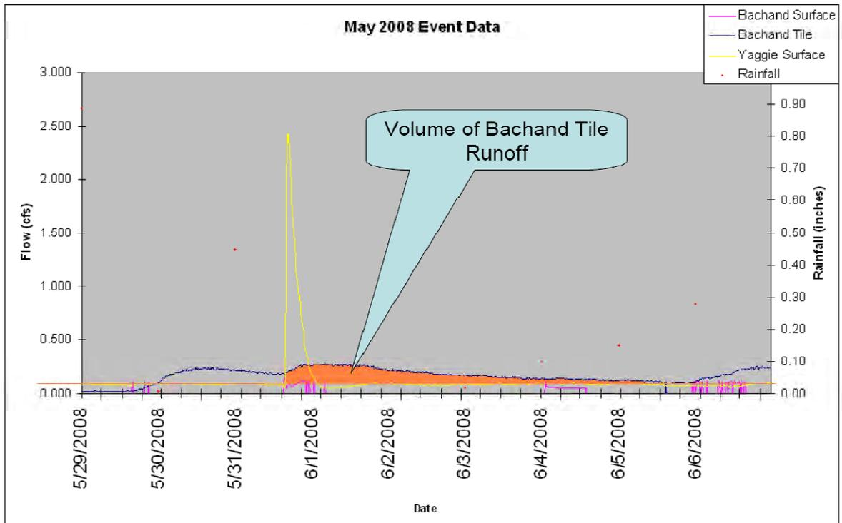
**Figure 71. Calculating runoff event volume for tile drainage**
